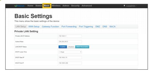
Under the Basic Settings, locate the MoCA tab to the far right of the selection. Ensure that MoCA Status is Enabled. If it is not, select the Enabled option. A list of additional options will appear after selecting "Enabled". Do not change these settings. Click "Save Changes" at the bottom.
